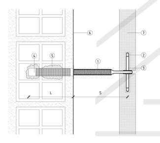
Load values are in kN for maximum deformation of 1,4 mm. These values relate exclusively to the flexural strength of this system made of stainless steel A2/A4.
